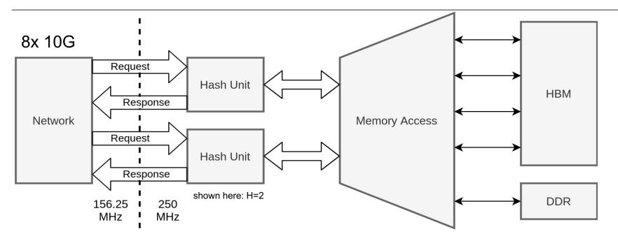
Simplified: Data hazard handling and out-of-order operations not shown [FPT 2021]
