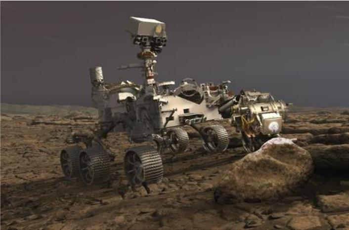
The Mars rover Perseverance illustrated here will carry a lunchbox-size PIXL device to analyze rocks and soil quickly in hopes of finding evidence of ancient life on the Red Planet. Virtex 5 accelerates specific stereo and visual tasks like image rectification, filtering, detection, and matching (NASA)
